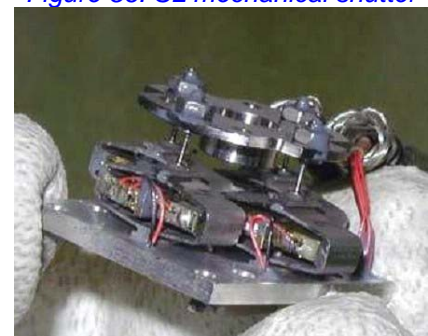
Figure 57: SL fiber optics injection mechanism
