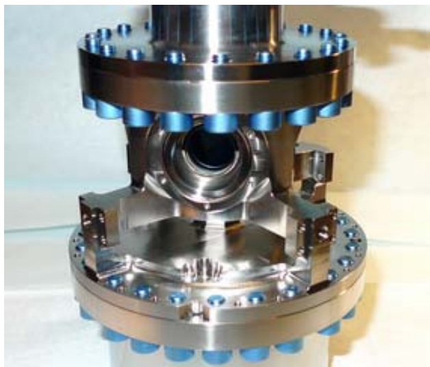
Figure 36: Selection chamber (Flight model )
