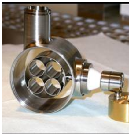
Figure 43: Ion pump developed for PHARAO
