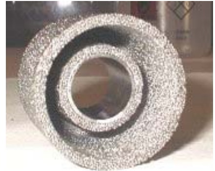
Figure 30: Porous titanium in which the caesium is stored
