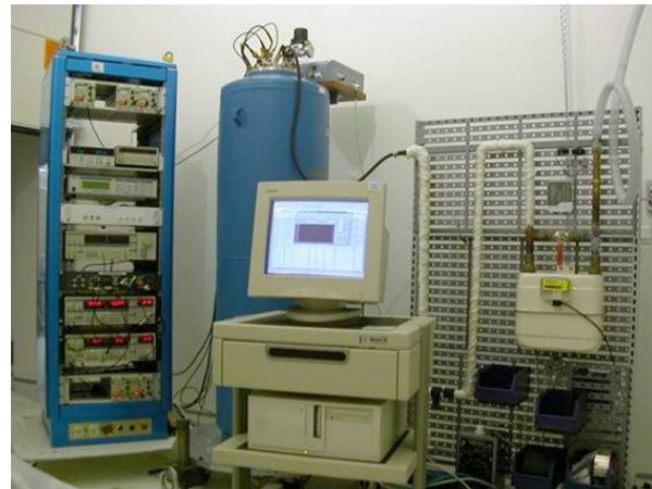
Figure 76: Cryogenic oscillator from UWA
