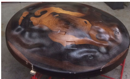
In production and finished self-heating mold for CNES
