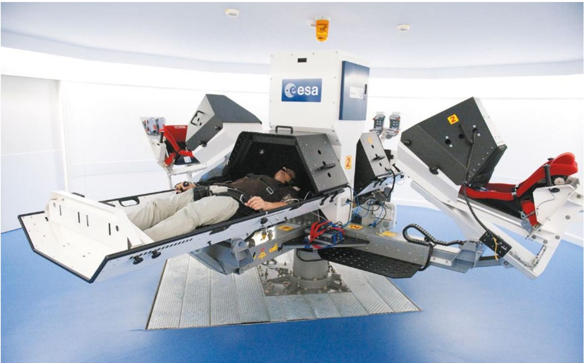
Since 2007, MEDES also has a short-arm centrifuge funded by ESA to gauge the effects of artificial gravity.
