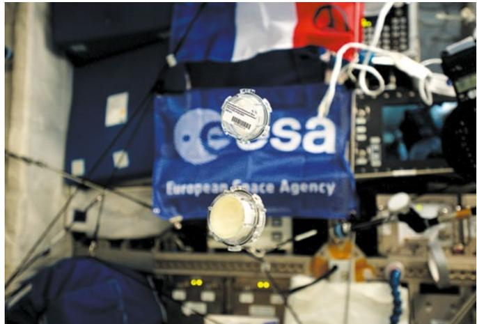
Shown here aboard the ISS, Aquapad is a new device for testing water quality on the station.
