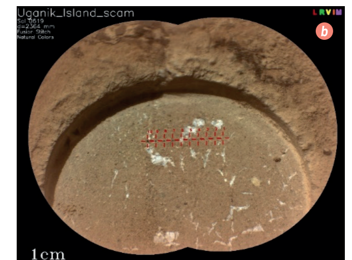
[b] - Analytical transect of laser shots (red crosses) in an abraded outcrop. From Maurice et al., Space Sci. Rev. The Mars 2020 Mission , 629-736, 2021.
