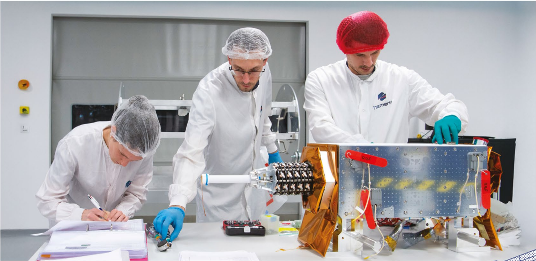
A nanosatellite from the Kineis constellation in the clean room at Hemeria.
