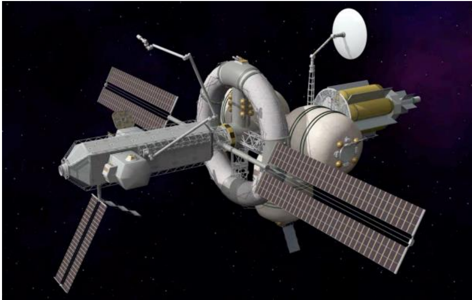
Figure 40: NASA's Nautilus-X is a multi-purpose platform that can accommodate a wide variety of missions. It integrates various propulsion platforms and life support systems along with guidance, navigation, and control systems (Henderson and Holderman, 2011).
