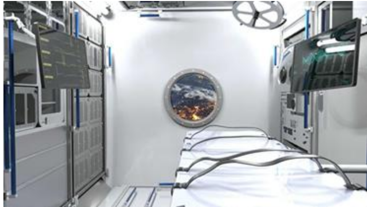
Figure 23: Representation of the simulated window in the SMC-LEO Module. Image Credit: Jeremy Battermann.
