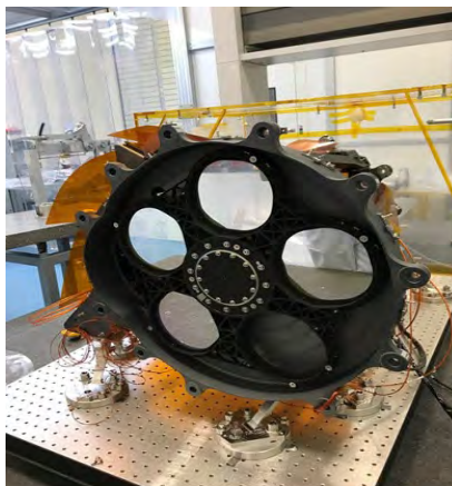
Grisms for NISP instrument (EUCLID Mission)
