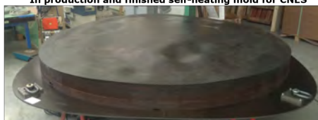
In production and finished self-heating mold for CNES
