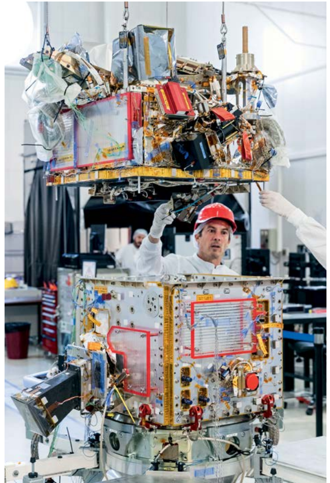
The Taranis payload is mated with its Myriade spacecraft bus in the clean room at the Toulouse Space Centre.
