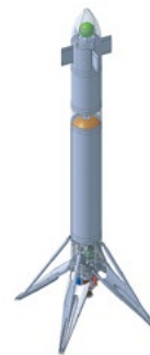
Standing only 13 metres tall and spanning 1.1 metres, Callisto will be a 'miniature' spacecraft.
