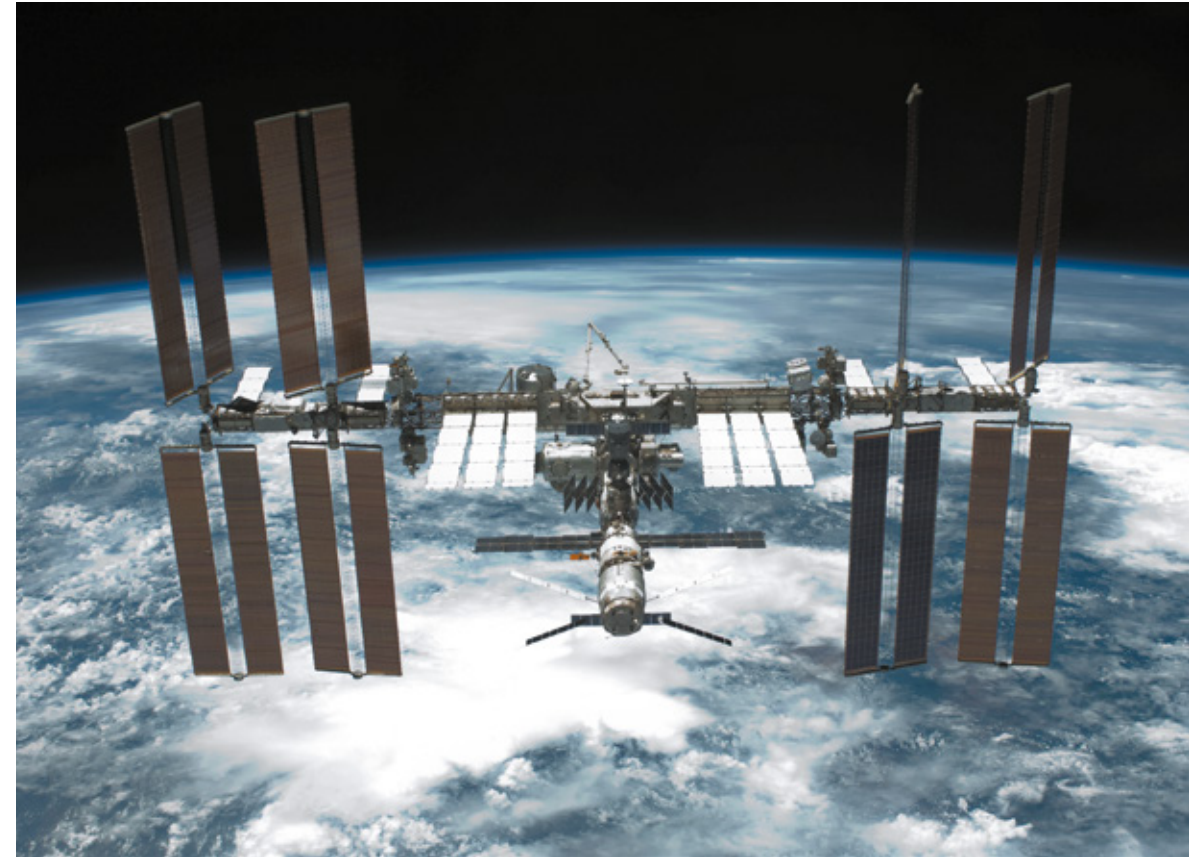
In the foreground, Europe's ATV-2 Johannes Kepler resupply vehicle berthed to the International Space Station.
