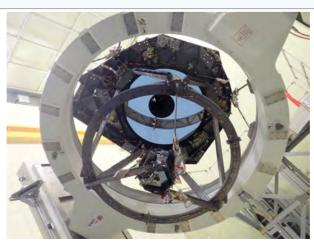
Euclid full-SiC telescope - Image courtesy of Airbus D&S
