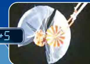
The order is given to separate the gondola from the envelope. The descent of the two mobile elements (envelope and gondola with its parachute) is monitored in real time down to the ground.
