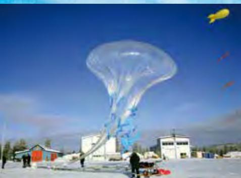
Stratospheric pressurised balloon (SPB) being released.
