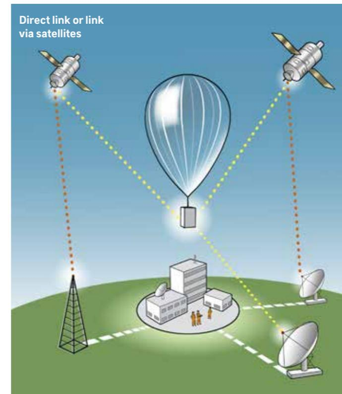
Balloons have gondolas which are constantly connected to a ground control centre. These gondolas are used to operate onboard actuators to release either gas or ballast. This makes it possible to control the ascent or descent of the balloon from the ground.
