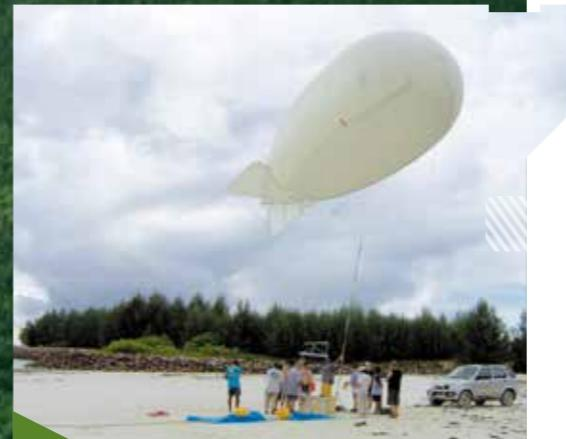
Launched in 2007, the Vasco programme brings together boundary layer pressurised balloons (BLPBs) and Aero-clippers. Objective: to gain a better understanding of the interactions between the atmosphere and the Indian Ocean.
