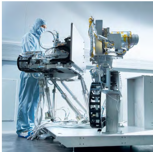
ZONDA Hexapod: Calibration of space optical instruments for MTG satellites Credits: Bertin Technologies
